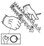
When the blades are correctly adjusted the play between the blades should be 0,2–0,4 mm, measured at the screws.
